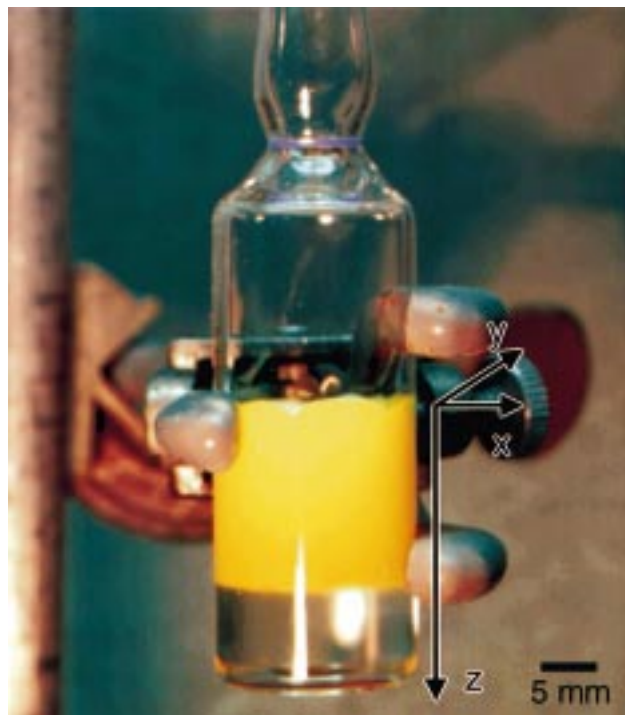
Figure 6. CdS mineralization of the \text{Cd}(\text{NO}_3)_2 doped hexagonal mesophase after 24 h of \text{H}_2\text{S} exposure. The hydrated \text{H}_2\text{S} enters the clear gel formed by the hexagonal mesophase from the top of the vial, and the opaque medium shows the z-position of the mineralization front.
